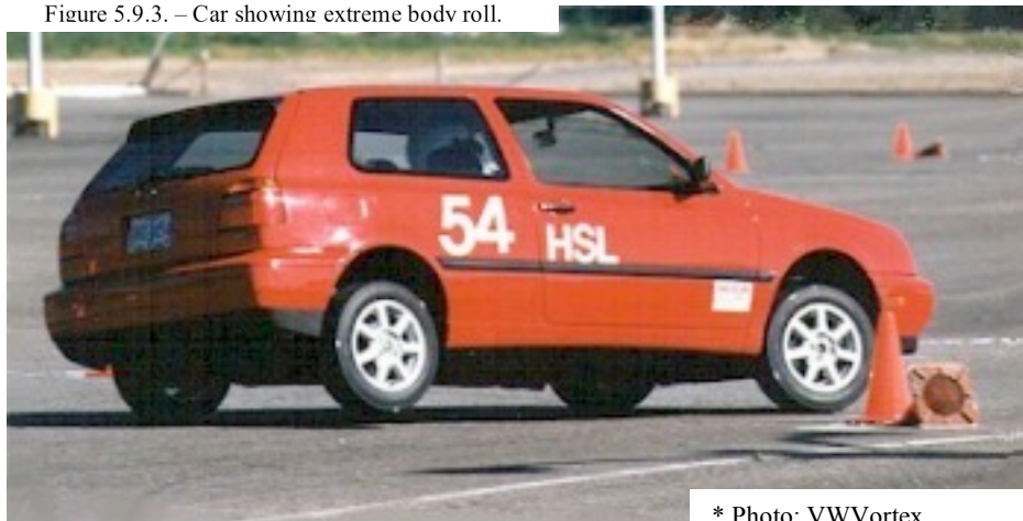
Figure 5.9.3. – Car showing extreme body roll.
