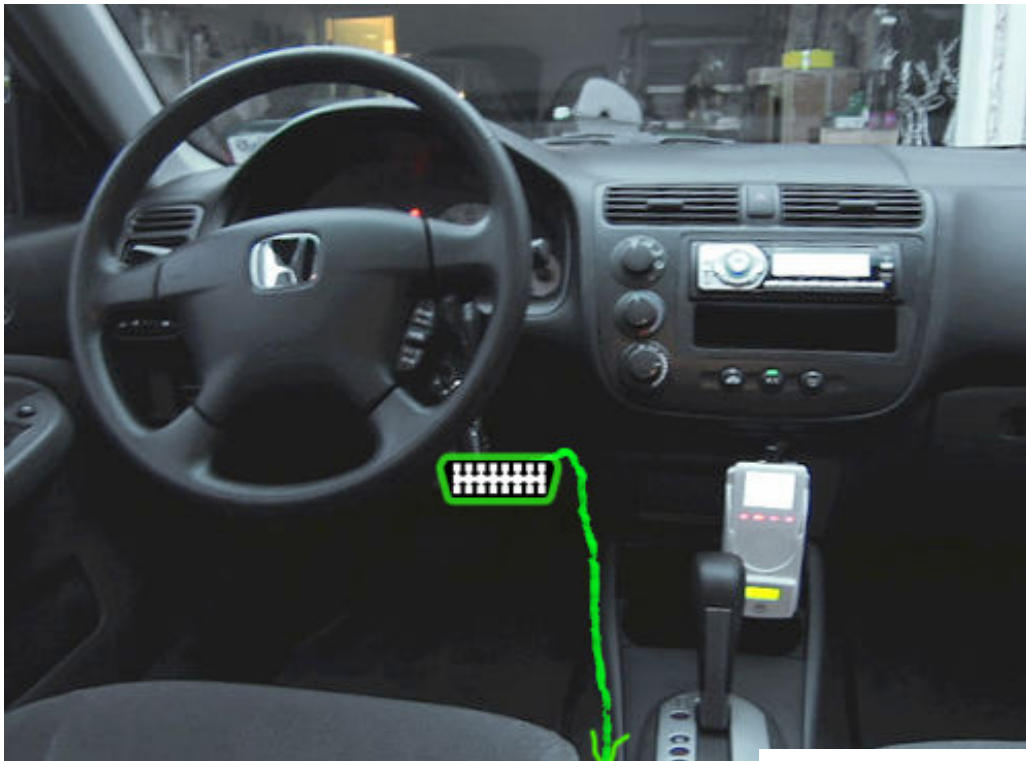
Figure 5.9.1. – Car interior showing OBDII port location.
